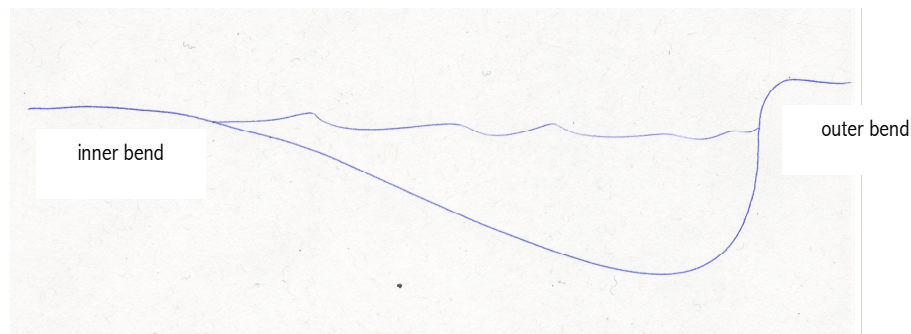
Figure 7. Comparing an Inner Bend and an Outer Bend (in cross-section)
